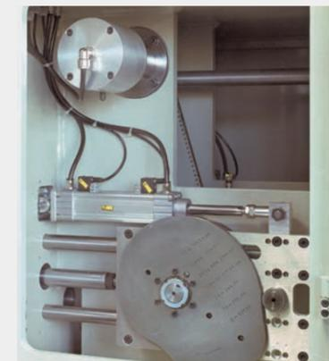
Cam housing with feed system
