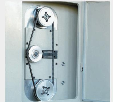
Cam drive with interchangeable pullers
